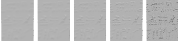
Figure 8: Back-projecting the mesh of a single scan of a fine-scale object (engravings are around 0.1mm deep). From left to right: mesh built after 4 scale space iterations; back-projection to levels 3, 2, 1 and 0 (final mesh).
