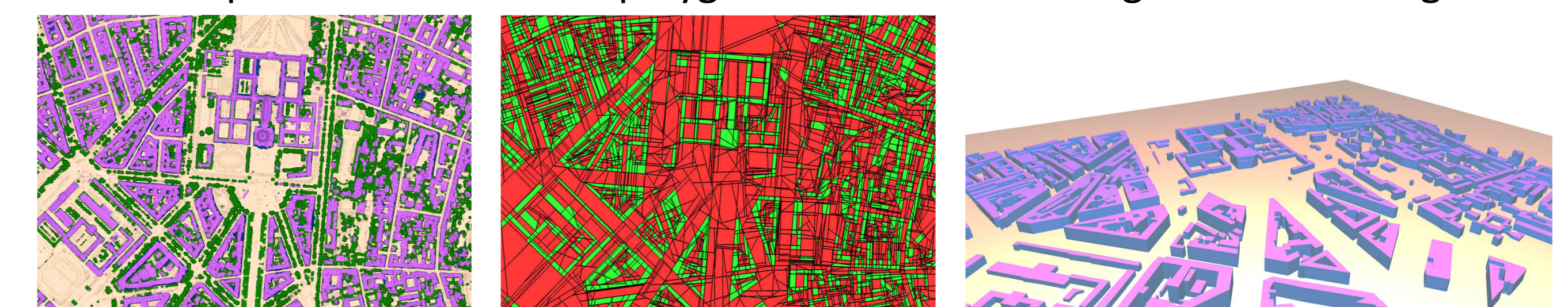
Classified input point cloud Labeled polygonal partition Output 3D model
