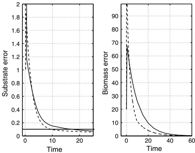
**Fig. 5** In *plain line* the biomass error and the substrate error of the asymptotic observer; in *dash line* of the hybrid bounded observer
