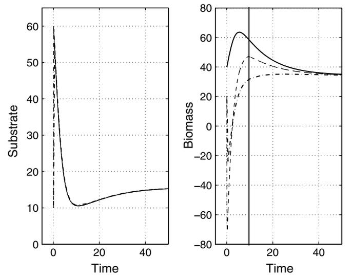
**Fig. 4** In dash line the hybrid bounded observer, in dash-dotted line the asymptotic one, in plain line the model
