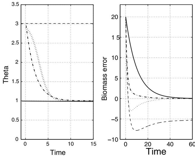
**Fig. 3**  $\theta$  values and biomass error for  $\theta=1$  in plain line, for  $\theta=3$  in dash line, for  $\theta$  time dependent in dotted line and in dash dotted line
