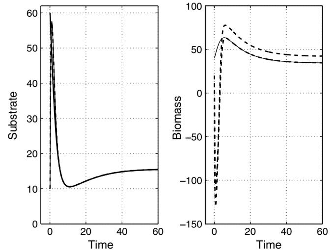
**Fig. 1** In dash line the high gain observer when the growth rate is partially known (bold) and when the model is perfectly known, in plain line the model
