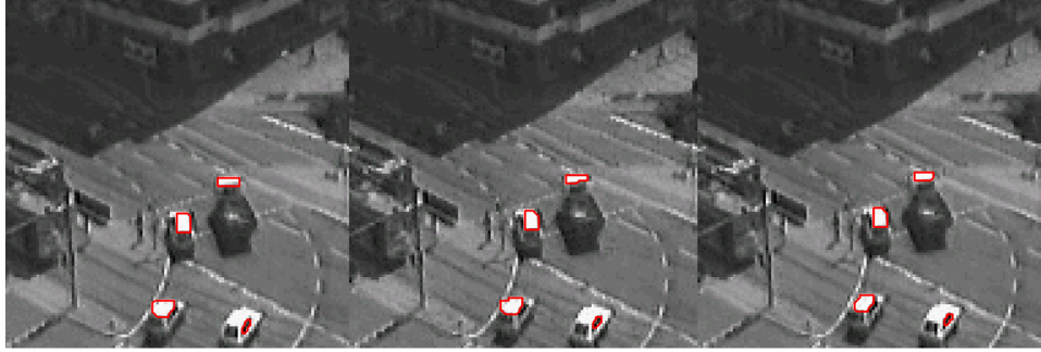
FIGURE 24. The images show three consecutive frames of a motion sequence of images. The boundaries are shown in red.
