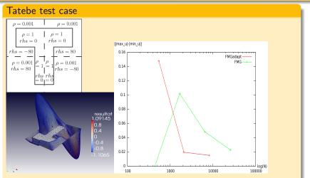
This test case is symmetric. After convergence, the difference between the maximum and the minimum must be equal to 0. We observe this difference decrease more quickly with adaptation.
