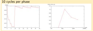
Converged solution, solution for 10 cycles per phase and difference between the two solutions.
