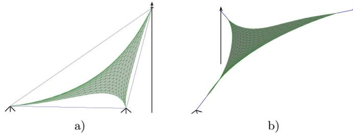
**Fig. 11.** Two modeling examples of membrane structures by using the triangular trimmed surfaces on minimal surface  $r_1(u, v)$  with  $a_1 = i_1 = 50$
