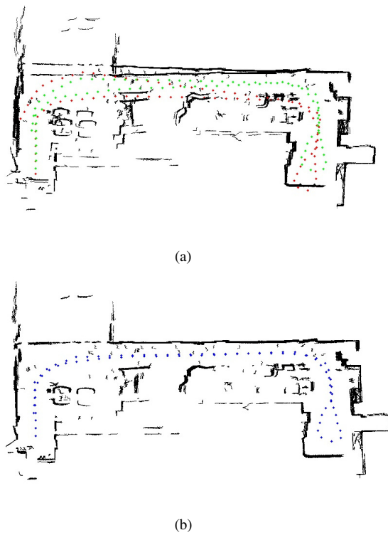
Fig. 5. 2D global maps obtained with the same laser data. 5(a) Map with EPSM pose estimation. 5(b) Map with spherical pose estimation.
