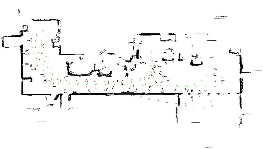
Fig. 5. Global map obtained by SLAM together with the original and recomputed position of the robot at several key instants.
