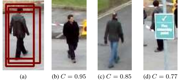
Figure 4: Confidence computation : (a) set of candidates for one person; (b) : a perfectly detected individual with a high confidence; (c) : an uncertain detection with an average confidence ; (d) : a bad detection with a low confidence due to occlusion.
