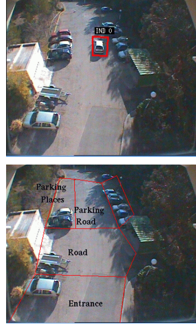
Figure 1. (a) Visualization of the event 'vehicle on the parking road'. (b) Manually defined zones in the scene.
