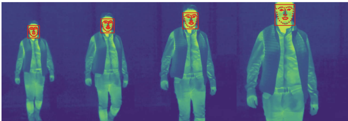
Figure 7: Monitoring system with thermal sensor. TFLD method applied on video sequence captured in the wild. A person, approximately 14m away, walks towards the camera while TFLD is tracking face and landmarks.
