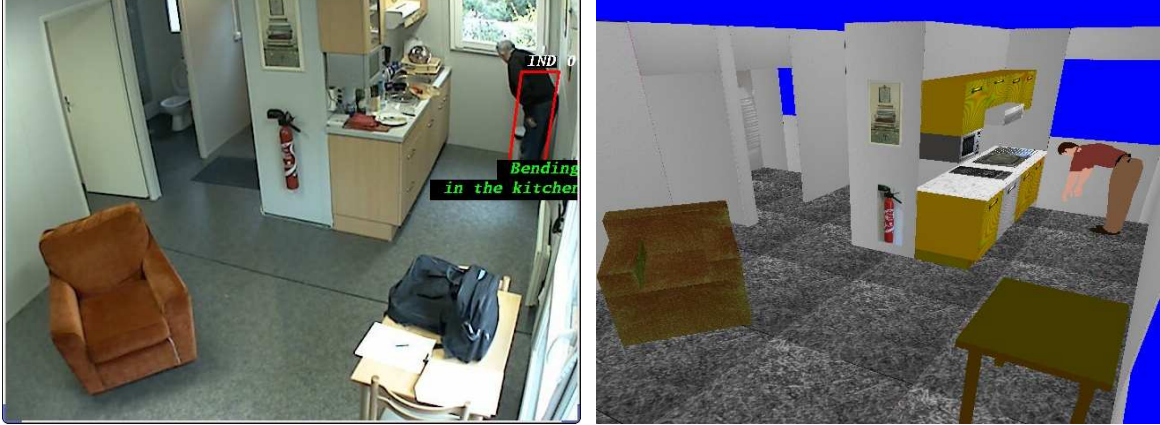
Fig.6. 2D and 3D visualization of the recognition of "bending in the kitchen" activity
