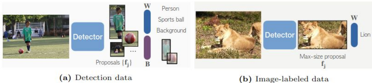
Fig. 3: Approach Overview. We mix train on detection data and image-labeled data. When using detection data, our model uses the standard detection losses to train the classifier ( W ) and the box prediction branch ( B ) of a detector. When using image-labeled data, we only train the classifier using our modified classification loss. Our loss trains the features extracted from the largest-sized proposal.
