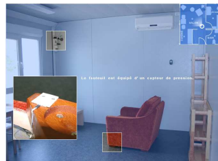
Pressure sensor underneath the legs of armchair
