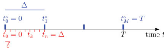
Figure A.2. The observation instants are t_k^o = k \Delta with \Delta = \frac{T}{M} ; the time-discretization instants are t_k = k \delta with \delta = \frac{\Delta}{n} for n given.
