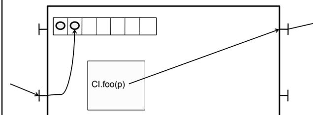
Primitive components communicating by *asynchronous* remote method invocations on interfaces (*requests*)
