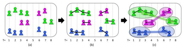
**Fig. 1**. The overview of the tracking approach in T frames: (a) The raw detection results; (b) the results of the short-term tracking; (c) the results of linked trajectories using online discriminated appearances.
