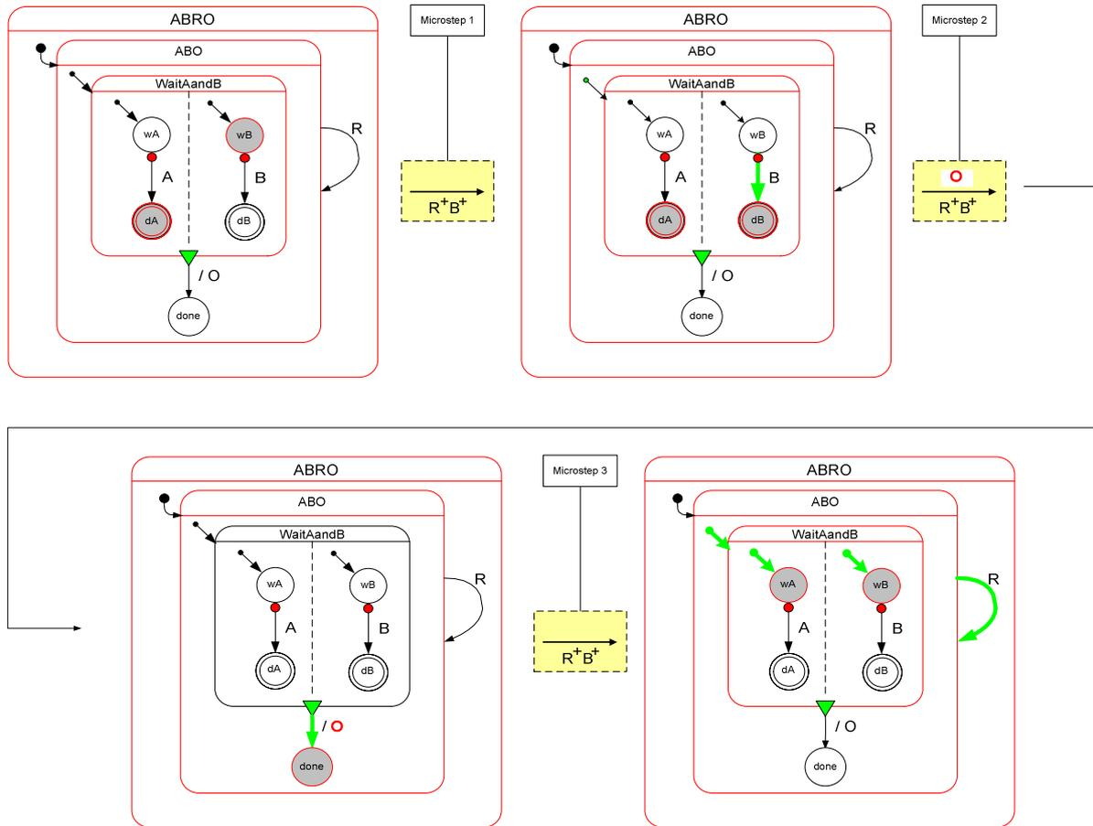
Figure 5-15: Microsteps in a case of weak abortion.
