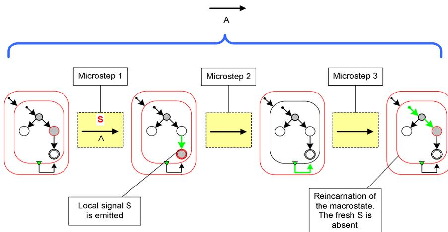
Figure 8-24: The microsteps of the third reaction.
