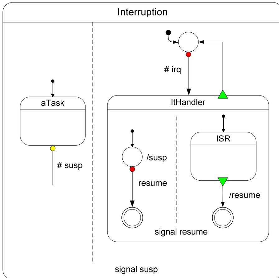
**Figure 8-6: Interruption Mechanism.**
