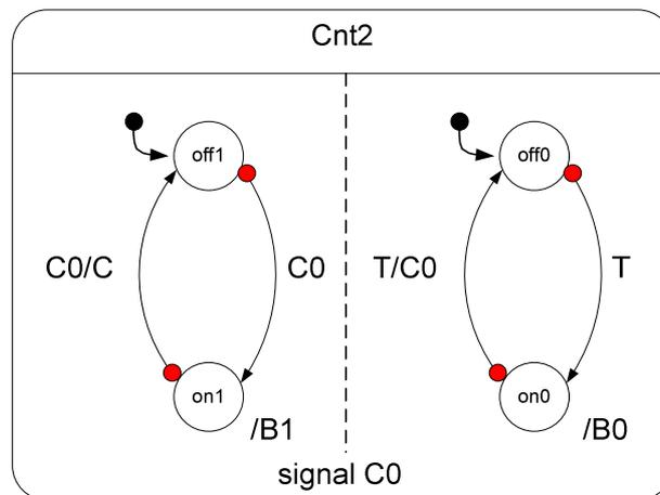
**Figure 5-3: SyncChart for a 2-bit binary counter.**
