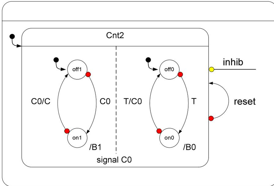
**Figure 8-5: 2-bit Counter with Suspension and Reset.**
