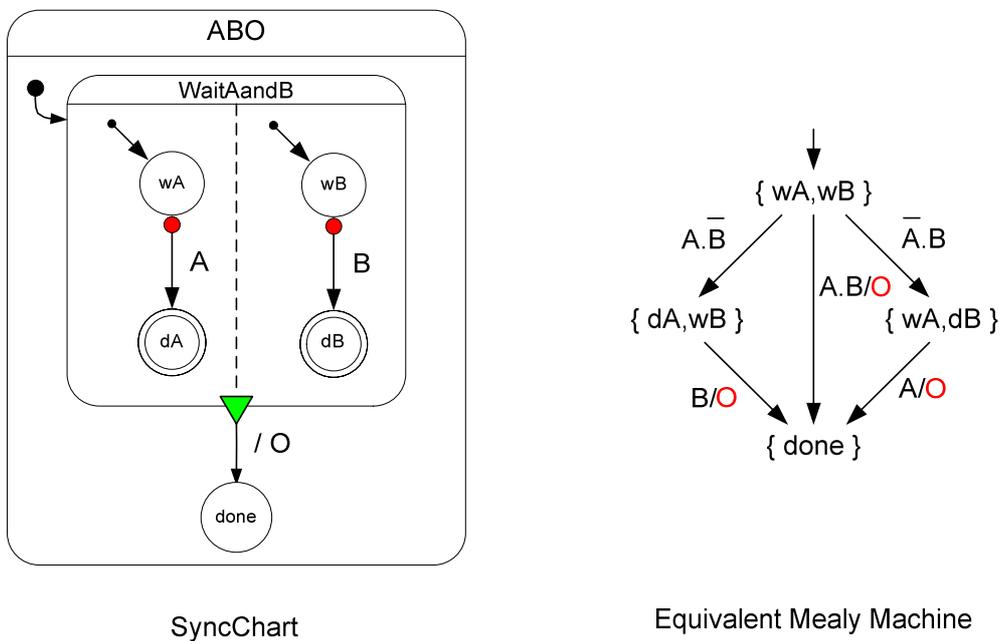
Figure 5-9: Synchronized Termination.
