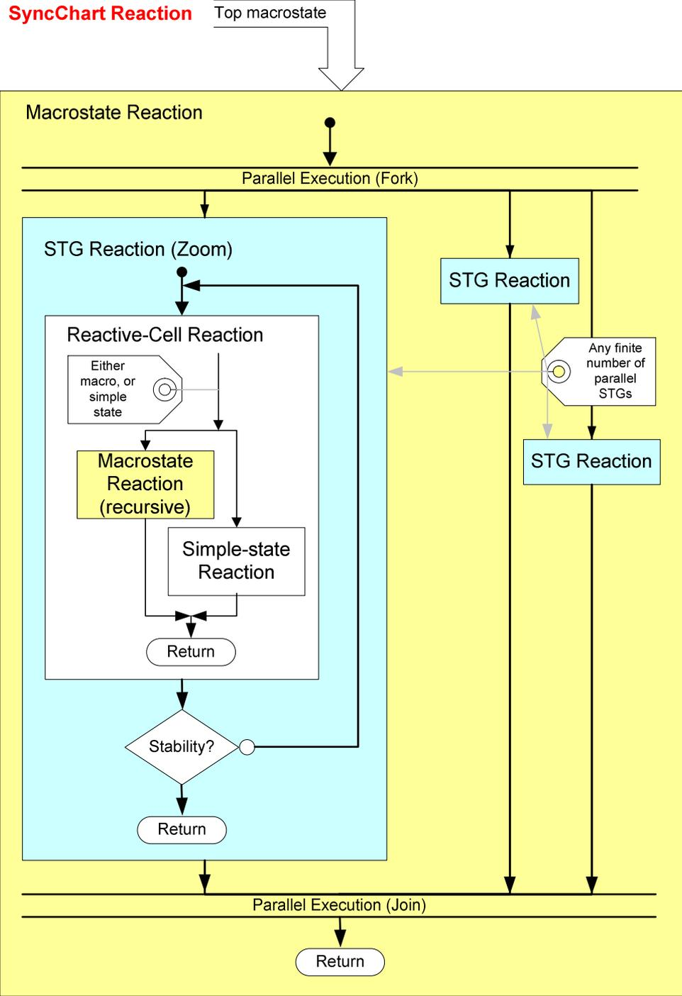
Figure 6-5: Overview of a Reaction.
