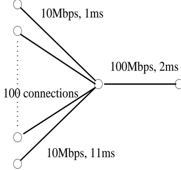
Figure 1: N persistent TCP connection sharing a single bottleneck link.
