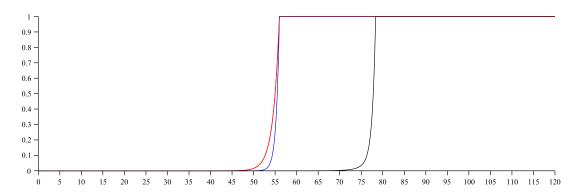
Figure 1: Upper bound on adversarial advantage (proven security) verses  $\log_2 q$  (where q=number of queries) for the cascade construction, assuming key length k = 56 and block length n = 64. Single encryption is the leftmost curve, double encryption is the middle curve [3], and triple encryption in the rightmost curve, as given by Theorem 4.
