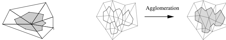
Fig. 1 Left: finite-Volume partition built as dual of a triangulation. Right: Greedy Algorithm for finite-volume cell agglomeration: four fine cells (left) are grouped into a coarse cell
