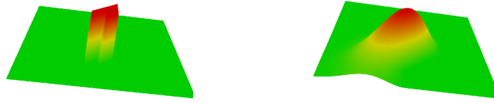
Fig. 2 Left: characteristic coarse grid basis function. Right: smooth coarse grid basis function
