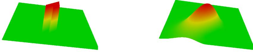
Figure 2. Left: characteristic coarse grid basis function. Right: smooth coarse grid basis function
