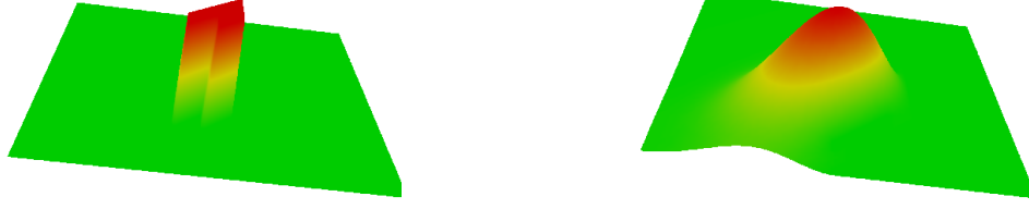
Figure 1: Left: characteristic coarse grid basis function. Right: smooth coarse grid basis function.
