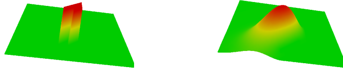
Fig. 2 Left: characteristic coarse grid basis function. Right: smooth coarse grid basis function
