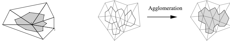
Fig. 1 Left: finite-Volume partition built as dual of a triangulation. Right: Greedy Algorithm for finite-volume cell agglomeration: four fine cells (left) are grouped into a coarse cell
