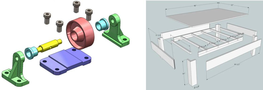
**Figure 1:** Manufactured objects are often created by assembling many parts, such as plates, wheels and tubes in mechanical assemblies (left) or planks in furniture assemblies (right). Objects are easier to fabricate and repair if they are made of standard parts also present in other assemblies.
