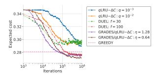
Fig. 7: Expected cost  $\mathcal{C}(\cdot)$  incurred by the different policies under the trace *Synthetic* in table I:  $q\text{LRU-}\Delta C$  ( $q=10^{-3},10^{-2}$ ), DUEL , GREEDY, and GRADES ( $\eta=1.28,0.64$  grafted with p=1 and  $q=10^{-3}$ ). Cache size k=313.
