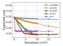
Fig. 6: Effect of grafting parameter p on the expected cost  $\mathcal{C}(\cdot)$  in a dynamic setting for  $\text{GRADES}/q\text{LRU-}\Delta C$  ( $\eta=0.64$ ). The cache is initialized to a stationary configuration as in Fig. 3. Now, only requests corresponding to region B from the synthetic trace are made. Cache size k=313.
