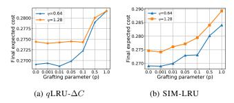
Fig. 5: Effect of the grafting parameter p on the final expected cost  $\mathcal{C}(\cdot)$ . GRADES/qLRU- $\Delta C$  ( $q=10^{-2}$ ) and GRADES/SIM-LRU for different learning rates under the trace *Synthetic* in Table I. Cache size k=313.
