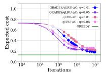
Fig. 8: Expected cost  $\mathcal{C}(\cdot)$  incurred by the different caching policies for the trace  $360^{\circ}$  *videos* in Table I. GRADES/*q*LRU- $\Delta C$  (q=0.01,0.05) with  $\eta=1.0$  and *q*LRU- $\Delta C$  (q=0.01,0.05). Cache size k=4000.
