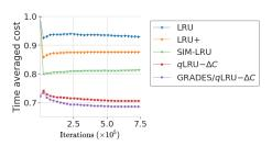
Fig. 9: The time averaged cost incurred by different policies under the trace Amazon trace: LRU, LRU+, SIM-LRU,  $q\text{LRU-}\Delta C \ (q=10^{-3})$  and GRADES/ $q\text{LRU-}\Delta C \ (\eta=6.9\times$  $10^2$ , grafted with p = 1). The level of approximability is 10%. Cache size k = 100.
