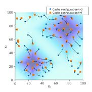
Fig. 1: Cached objects' movements in the representation space  $(\mathbb{R}^2)$  during [0,T] when the cache is managed by GRADES. The catalog is made by the points in a  $100 \times 100$  grid, dark shaded areas correspond to more popular objects. Dissimilarity cost  $C_d(x,y) = 1/10||x-y||_1$ , retrieval cost  $C_r = 1$ , cache size k = 50. See the description in Sect. V.
