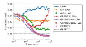
Fig. 4: Expected cost  $\mathcal{C}(\cdot)$  incurred by different policies under the trace *Synthetic* in Table I: LRU+, SIM-LRU, qLRU- $\Delta C$  ( $q=10^{-2}$ ), GREEDY, and GRADES ( $\eta=0.64$ , plain and grafted with  $p=10^{-1}$ ). Cache size k=313.
