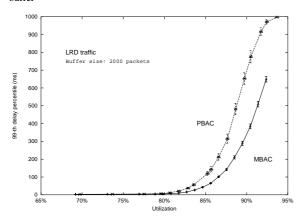
Fig. 6. Delay performance vs link utilization, using a 2000 packets buffer
