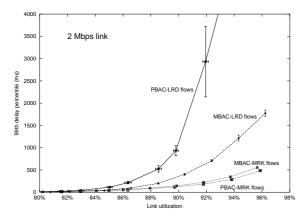
Fig. 4. Delay performance vs link utilization (2 Mbps link)
