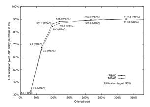
Fig. 3. Link utilization vs offered load
