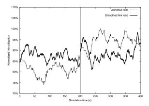
Fig. 2. Measurement-Based Admission Control operation
