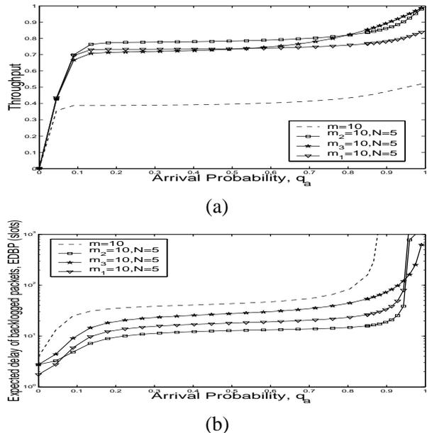
Fig. 2. (a) and (b) show the throughput and delay of backlogged packets. The objective under all the schemes is to maximize the throughput. The number of mobiles is 10 and the number of levels is 5.
