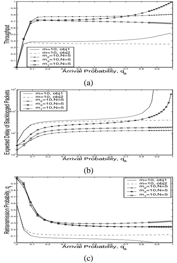
Fig. 4. (a), (b) and (c) show the throughput, EDBP and retransmission probabilities. The objective under schemes 1-3 is to minimize EDBP ( $obj_2$ ). The number of mobiles is 10.
