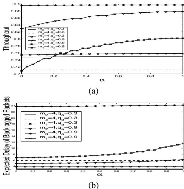
Fig. 10. (a) and (b) show throughput and delay of backlogged packets when the multi-criteria objective is optimized for  $N = 5$ .
