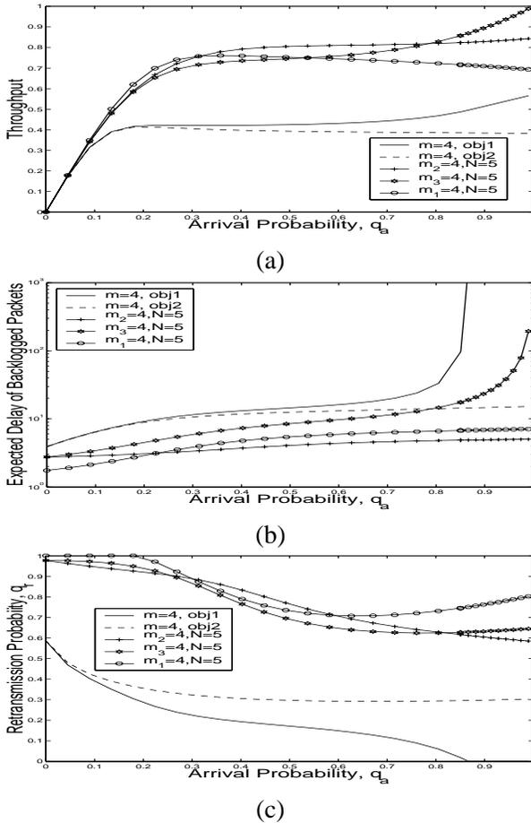
Fig. 3. (a), (b) and (c) show the throughput, EDBP and retransmission probabilities. The objective under schemes 1-3 is to minimize EDBP ( $obj_2$ ).  $m, m_1, m_2$  and  $m_3$  refer to standard Aloha, schemes 1, 2 and 3 respectively. The number of mobiles is 4.  $obj_1$  refers to the objective of maximizing the throughput.
