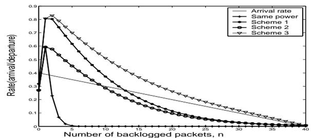
Fig. 7. Stability and instability of slotted Aloha schemes : The arrival probability  $q_a = 0.01$ , number of mobiles  $m = 40$ , number of levels  $N = 5$  and retransmission probability  $q_r = 0.8$ .
