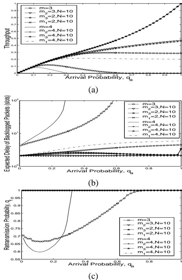
Fig. 13. (a), (b), (c) show the throughput, EDBP and retransmission probability when the objective is to minimize the delay of backlogged packets for all the schemes for 3 and 4 mobiles.
