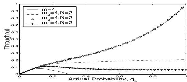
Fig. 14. Equilibrium throughput when the objective is to minimize the individual EDBP for all the schemes for 4 mobiles and  $N = 2$  levels.
