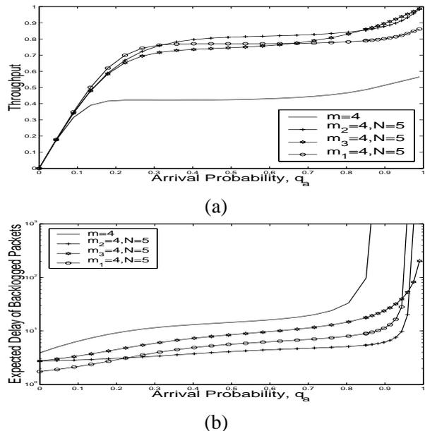
Fig. 1. (a) and (b) show the throughput and delay of backlogged packets. The objective under all the schemes is to maximize the throughput. The number of mobiles is 4 and number of levels is 5.
