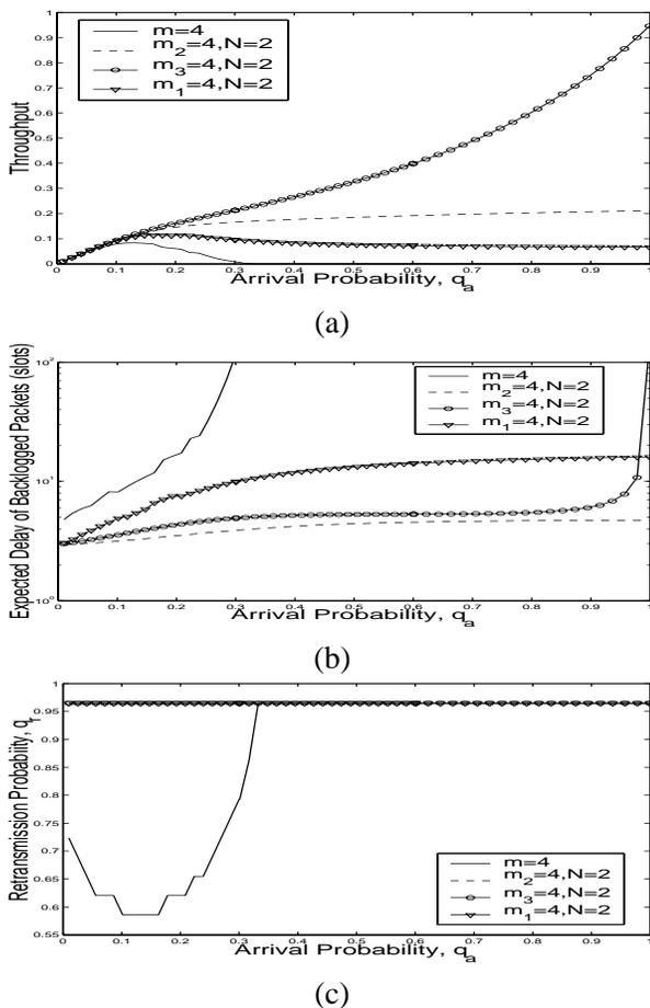
Fig. 12. (a) (b) and (c) show the throughput, EDBP and retransmission probability when the objective is to maximize the throughput for all the schemes for 4 mobiles and 2 levels.
