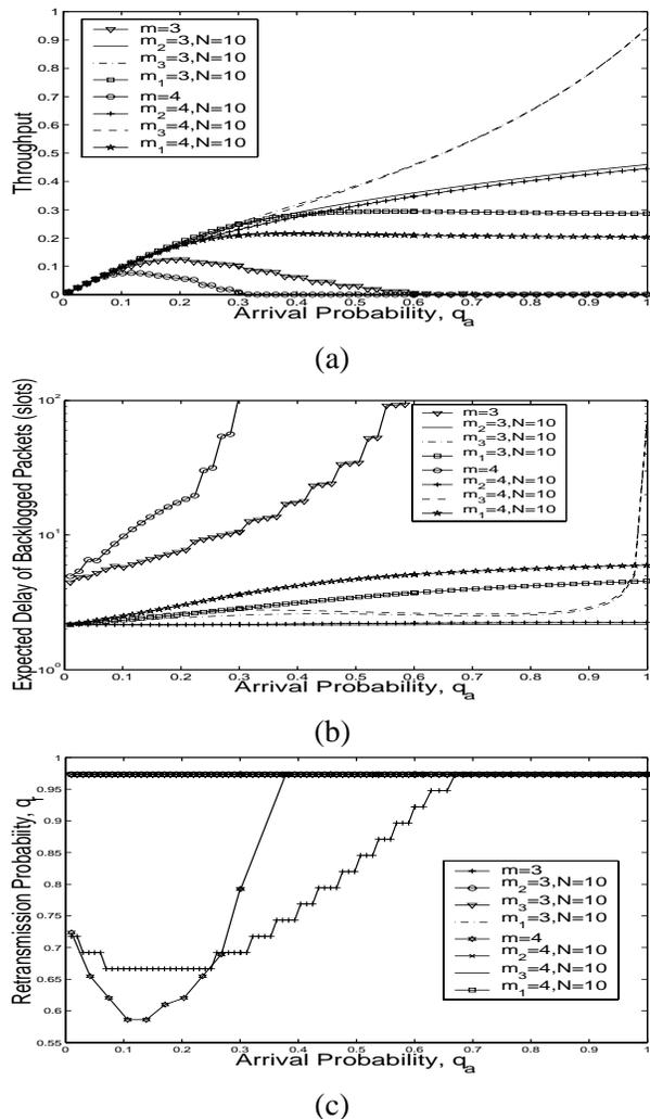
Fig. 11. (a), (b), and (c) show the throughput, EDBP and retransmission probability when the objective is to maximize the throughput for all the schemes. for 3 and 4 mobiles.
