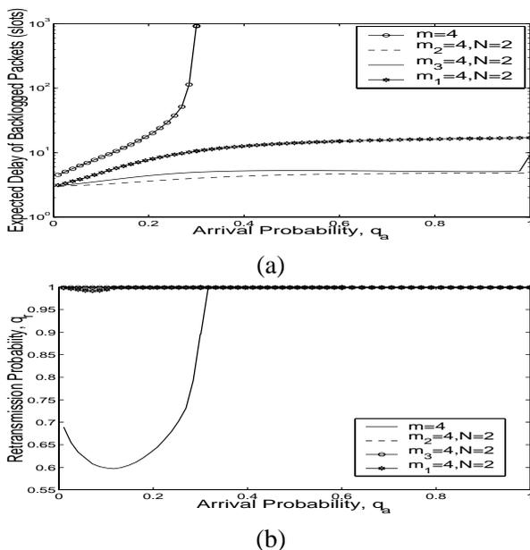
Fig. 15. (a) and (b) show the EDBP and retransmission probability when the objective is to minimize the EDBP for all the schemes for 4 mobiles and 2 levels.
