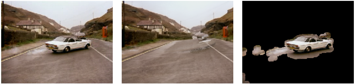
Fig. 2. Separation of background and mobile objects, car sequence #1. Original image (left), corresponding image from mosaic (middle), extracted mobile objects (right).
