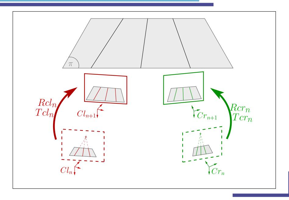
Features lying on the  $\pi$  plane have projections in 2 images constrained by the planar homography H<sub> $\pi$ </sub>:
