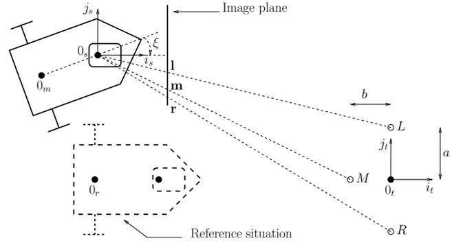
Fig. 2. Unicycle-like robot with a vision-based sensor
