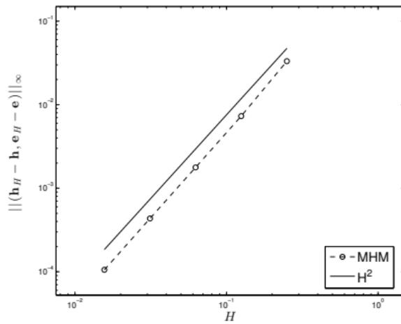
$\mathbb{P}_1$  elements for the edges,  $\mathbb{P}_3$  for the electromagnetic field, LF2 time-scheme.
