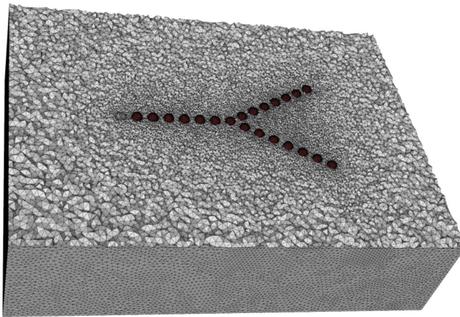
Y-shaped, 21 Au-nanospheres waveguide
