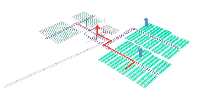
Computational setting of geological repository structures and its environment
