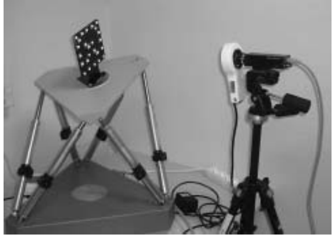
Fig. 16. Table of Stewart (DeltaLab) with vision system.
