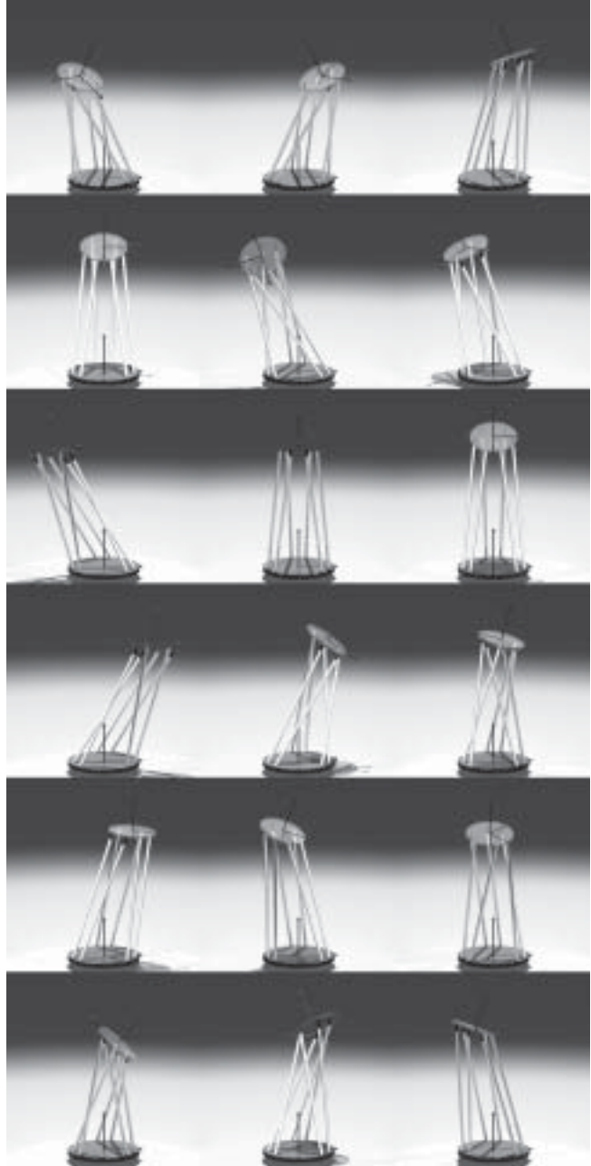
Fig. 13. Representation of the 18 poses of the Gough platform from the set \Upsilon_{s_4} .
