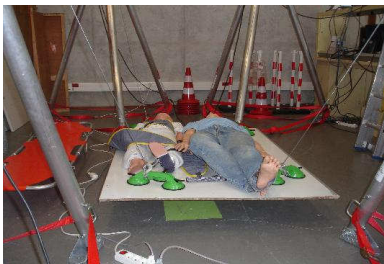
Fig. 5. Lifting of a 75kg mannequin and a 35 kg mannequin on a 25 kg platform.
