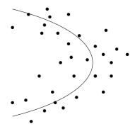
Bias due to curvature: more mass outside than inside projecting on a point where the curvature is large.
