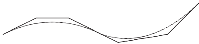
Figure 12: Linear, quadratic, and cubic B-spline curves sharing the same control polygon. The control polygon is equal to the linear B-spline curve. The curves are planar, i.e. the space dimension is two.
