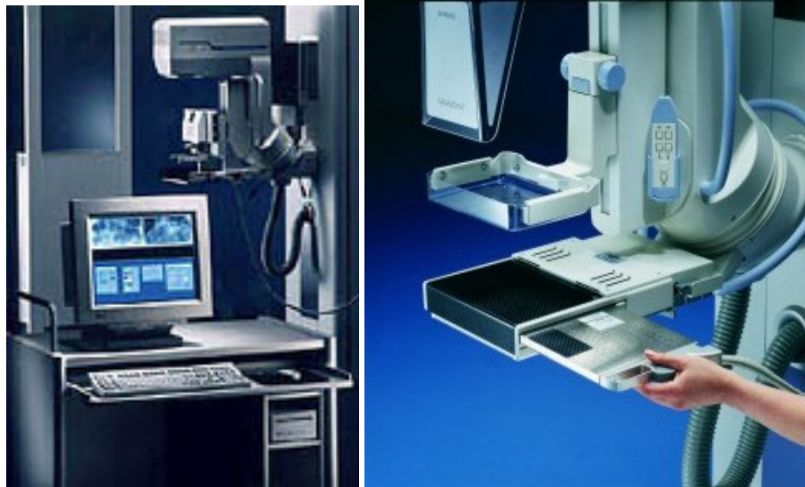
Figure 11: A soft copy environment produces digital mammograms, which are stored directly into a computer. This figure shows the Opdima System from Siemens, which was designed for near real-time computer guided biopsy.
