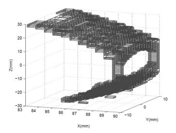
Fig. 13. Reachable workspace by topology  $H_1$ , given joint limit of  $[-30^{\circ}, 30^{\circ}]$ .
