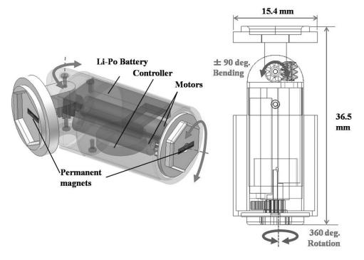
Fig. 8. Design of the heterogeneous module.
