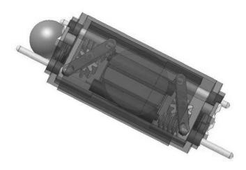
Fig. 15. New design of homogeneous bending module prototype, more compact with two motors per bending module. This allows bending actuation on both ends of the module.
