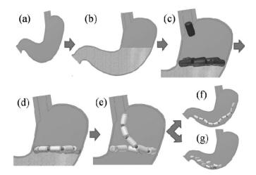
Fig. 2. The proposed procedures: (a) empty stomach, (b) stomach filled with a liquid, (c) ingested capsules on the liquid surface, (d) assembled modules, (e) robotic configuration and diagnosis/intervention, (f) reconfiguration to a snake-like topology, and (g) disassembled modules.
