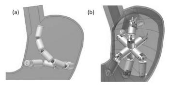
Fig. 1. Robotic schemes: (a) homogeneous scheme and (b) heterogeneous scheme for the endoluminal reconfigurable platform.
