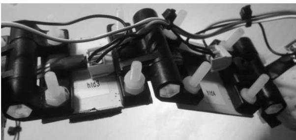
Fig. 2. Actual collar components: Plates with 4 reference points, connected by a hinge. The tips of the 4 screws are the 4 reference points
