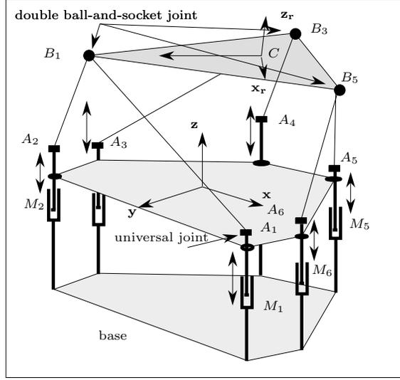
Figure 1: The parallel prototype: the prismatic actuators move the articulation point  $A_i$  along a vertical axis.
