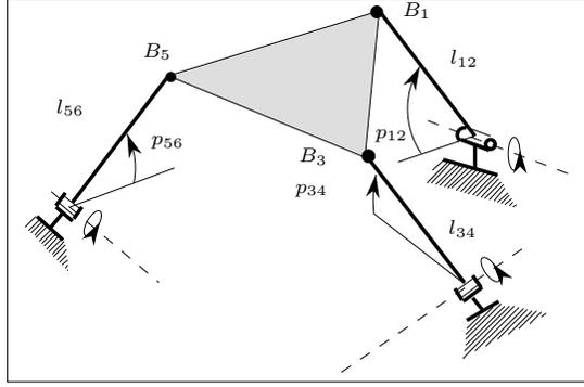
Figure 2: The equivalent mechanism of the INRIA prototype
