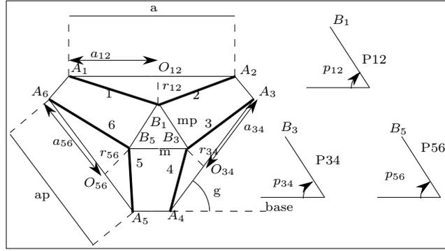
Figure 2: Notation (the TSSM is represented in top view)
