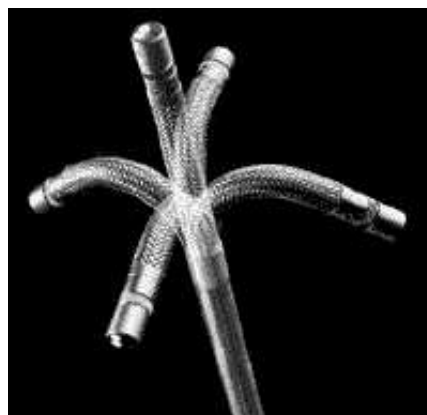
Fig. 1. The motion of the tip of an endoscope
