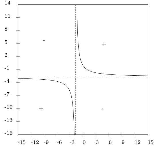
Figure 2. Singularity hyperbola and the sign of  $|J^{-1}|$  (for  $l_1 = 1, l_2 = 5, l_3 = 1, l_4 = 2$  and  $\theta = \pi/2$ )
