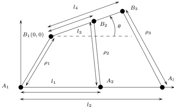
Figure 1. A special class of 3-RPR planar parallel manipulator
