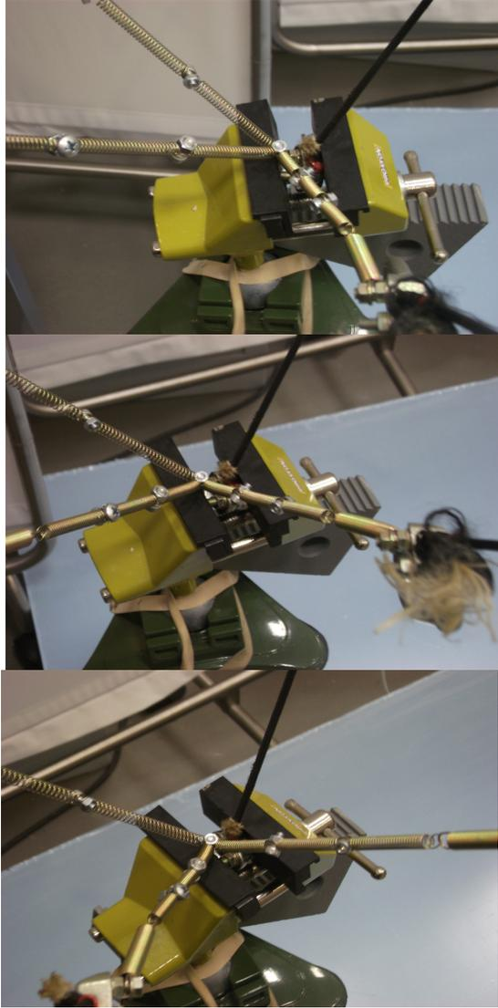
Fig. 4. An experiment with a 4-1 robot: we start in a configuration in which 3 wires are under tension (1,2,3), the fourth one being slack (top picture). Then we start decreasing the length of wire 4. At some point the tension in wire 3 is almost 0 (middle picture). Continuing decreasing the length of wire 4 leads to a pose in which the tension in wire 3 is 0 while wire 4 is becomes under tension (bottom picture).
