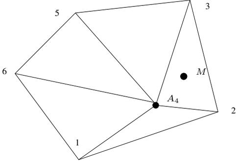
Fig. 2. If  $A_4$  lies inside in the convex hull of the  $A_i$ 's, then a decrease of  $\rho_4$  leads to a pose where only 3 wires are under tension (here wires 2,3,4)
