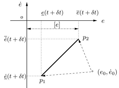
Fig. 3. Range of the next state in phase plane
