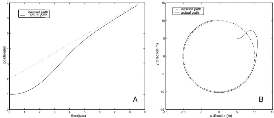
Figure 5: Tracking performance of the proposed algorithm with large  $A$  value,  $A=5$  instead of 1 in Fig. 5 and 6. A: Tracking a straight line; B: Tracking a circular path.
