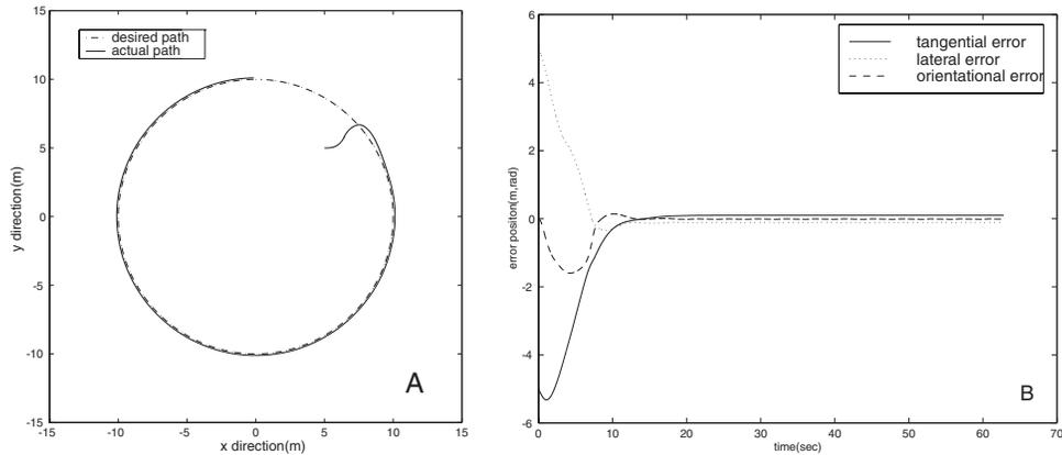
Figure 4: *Performance of the proposed algorithm. A: Control performance for tracking a circle path; B: Tracking errors.*
