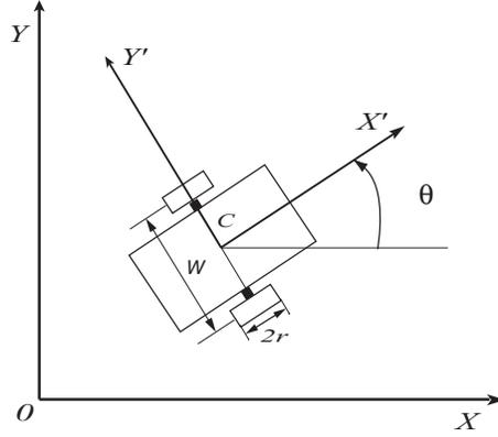
Figure 1: *Model of a wheeled mobile robot*
