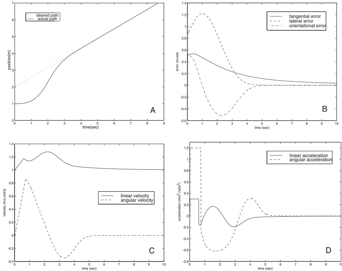
Figure 3: *Tracking a straight line. A: Tracking performance; B: Tracking errors; C: Velocities of the robot; D: Accelerations of the robot;*
