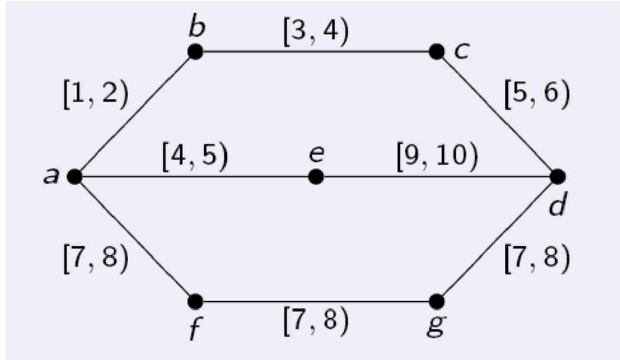
The interval(s) on an edge represent the period of time when it exists.
