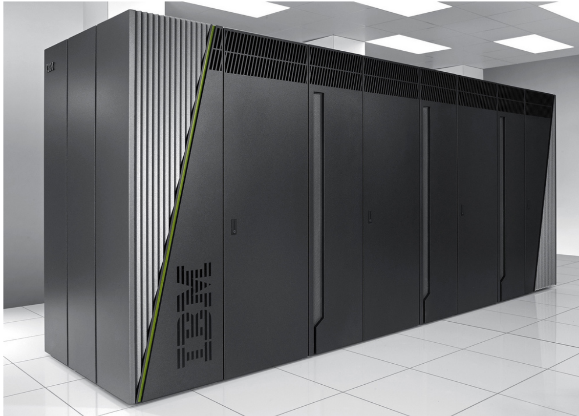
Sequoia system, Lawrence Livermore National Laboratory IBM BlueGene/Q, Power BQC 16C 1.6 GHz, custom interconnect 1572864, 20132 TFlop/s peak
