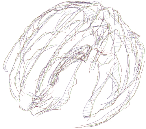
Figure 2. Registration of the mean lines set (in blue) towards one subject's lines set (in red). A unique deformation transports all the mean blue lines to the registered green lines. The spatial consistency constraint as well as the smoothing effect of the norm of currents prevents overfitted registrations from occurring. The residuals (i.e., the difference between the registered green lines and target's red lines) contains physical and numerical noise as well as possible non-diffeomorphic variations. They are considered here as noise: the statistics on brain shape will rely only on the diffeomorphism. A movie of this deformation can be seen at first author webpage: www-sop.inria.fr/asclepios/personnel/Stanley.Durrleman .
